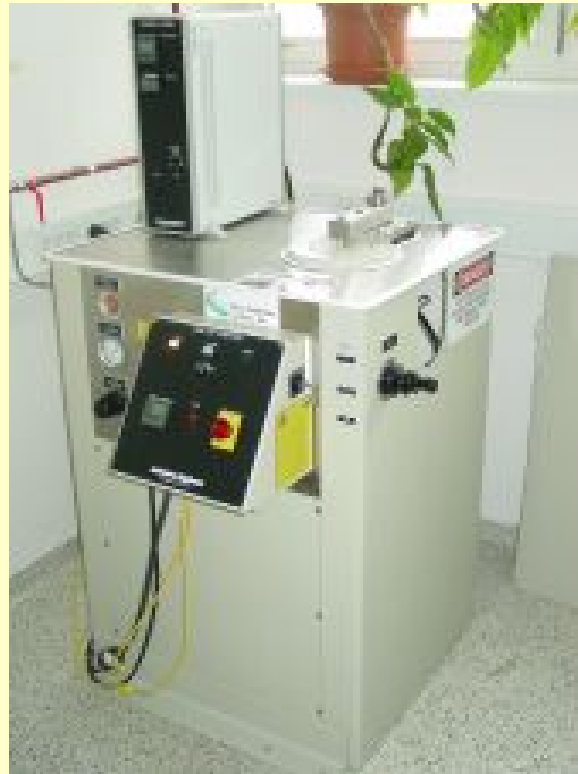
Warm Isostatic Press Max. pressure: 400 MPa Max. temperature: 80 °C Volume: 2,5 l
