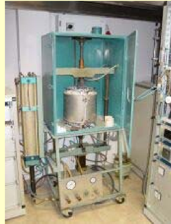
Hot press Max. temperature: 1250 °C Max. pressure: 100 MPa Max. diameter: 25 mm
