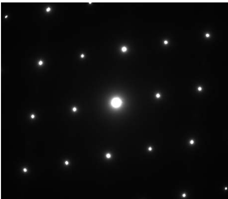
Fig. 17. Electron diffraction pattern with a low-indexed zone axis aligned almost parallel to the electron beam. Note that under that conditions the scattered intensity of the different spots is approximately the same.
