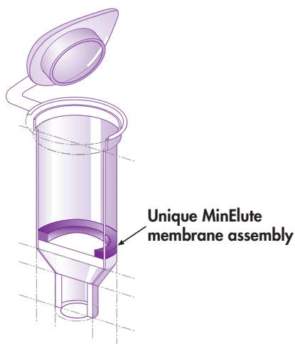
Figure 2. Unique membrane assembly enables low elution volumes. Cross-section of MinElute column.
