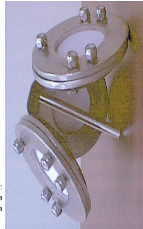
Fig. 1. Exploded view of a POCIS showing the sorbent layer contained between two membrane disks sandwiched between two support rings. A standard field deployed POCIS has an effective sampling surface area of 41 cm 2 .
