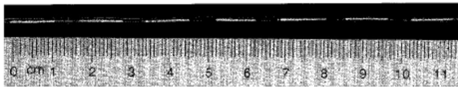
FIG. 1. High throughput flow cytometry. A : Schematic view of the flow cytometer, autosampler, and peristaltic pump. B : Adjacent samples of latex microspheres separated by air in the 0.02-in (254- \mu\text{m} ) ID tubing between the peristaltic pump and the flow cytometer.
