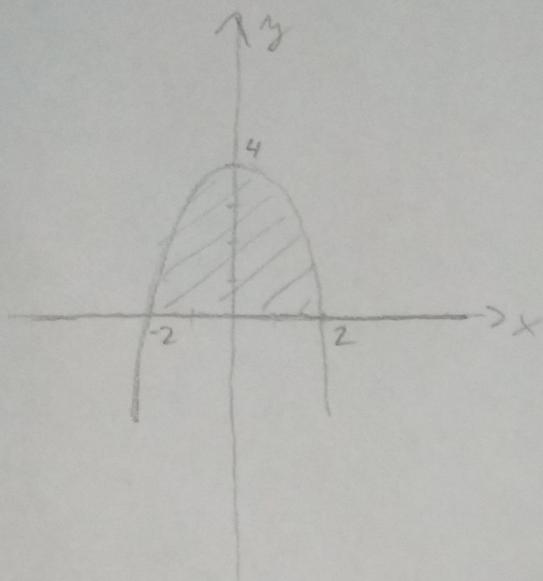
$$\begin{aligned} \int_{-2}^2 4 - x^2 - 0 \, dx &= 4 \int_{-2}^2 1 \, dx - \int_{-2}^2 x^2 \, dx = \\ &= [4x]_{-2}^2 - \left[ \frac{x^3}{3} \right]_{-2}^2 = \\ &= 8 - (-8) - \left( \frac{8}{3} - \left( -\frac{8}{3} \right) \right) = 16 - \frac{16}{3} = \\ &= \frac{48}{3} - \frac{16}{3} = \underline{\underline{\frac{32}{3}}} \end{aligned}$$
