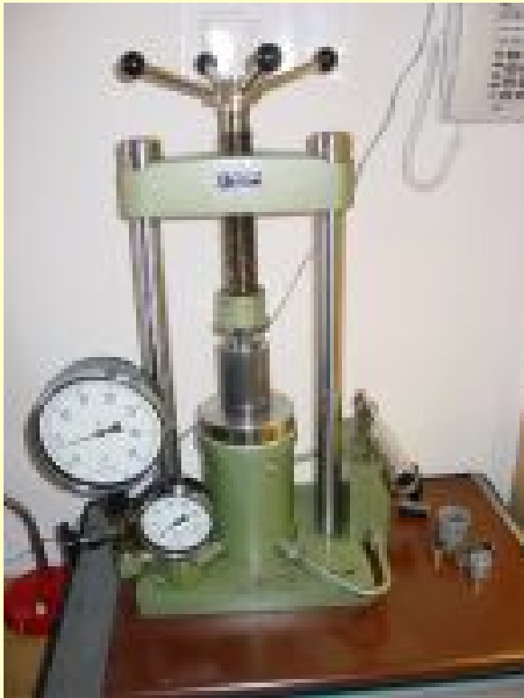
Hydraulic Uniaxial Press Maximum pressure: 120 MPa
