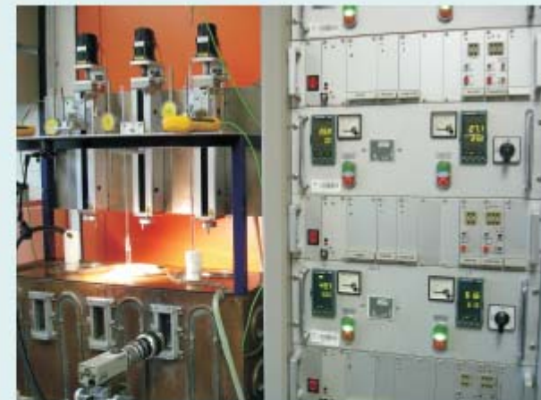
A view of vapor growth equipment
