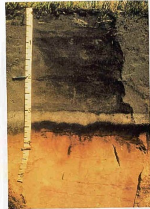
Photo 10.—A soil that has a plaggan epipedon about 90 cm (3 ft) thick. The soil presumably came from the heath. Variations caused by mixing of materials can be seen. This soil unit has straight boundaries, and it is lighter than the surrounding landscape. Plaggan epipedons are not known to occur in the United States but are common in parts of Western Europe.
