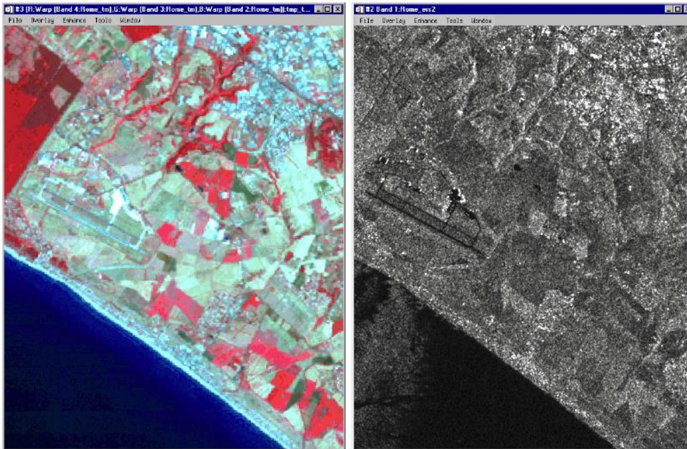
Figure 12-1: Landsat TM False-color Infrared Composite (bands 4, 3, 2 as RGB), left. ERS-2 SAR Data, right
