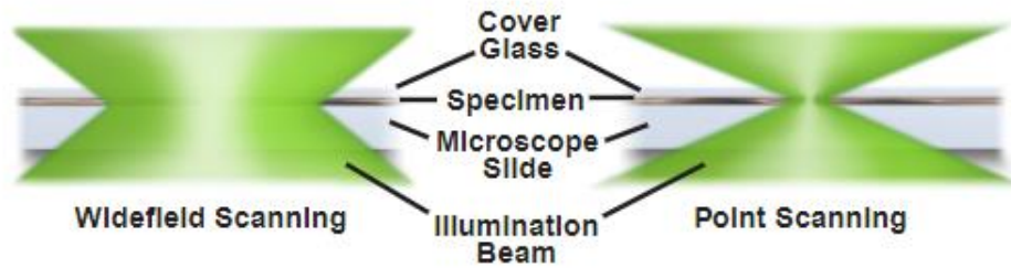
Figure 2 - Widefield Versus Point Scanning of Specimens
