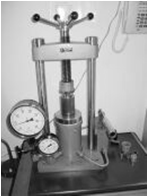
Hydraulic Uniaxial Press Maximum pressure: 120 MPa
