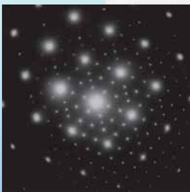
The basic operations of the TEM imaging system involve (A) projecting the diffraction pattern on the screen. In each case the intermediate lens selects either the back focal plane or the image plane of the objective lens.
