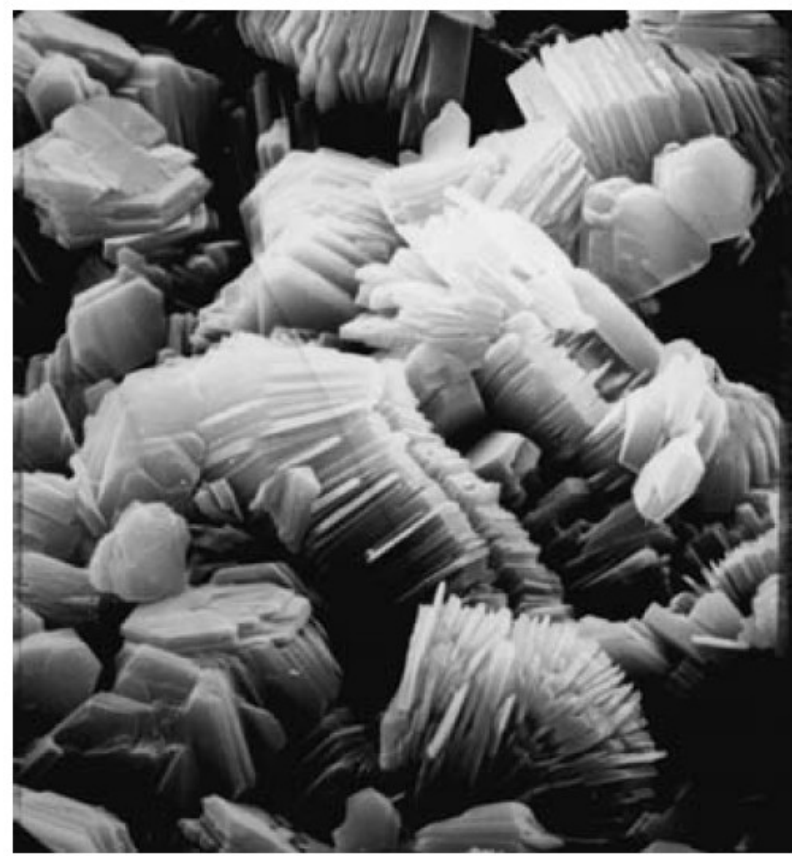
Electron microscope photograph of kaolinite clay minerals magnified 4700 \times . Note the flake-like appearance.
