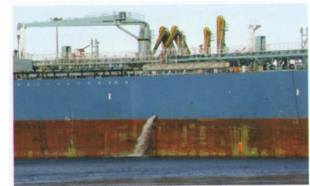
Figure 2. Release of ballast water. Photo: S. Olenin.
