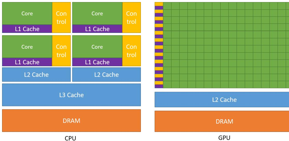
The GPU contains a large number of GPU computing cores that are organized into groups (SM, streaming processors). The GPU performs computational operations on a group of data - vector data processing.
