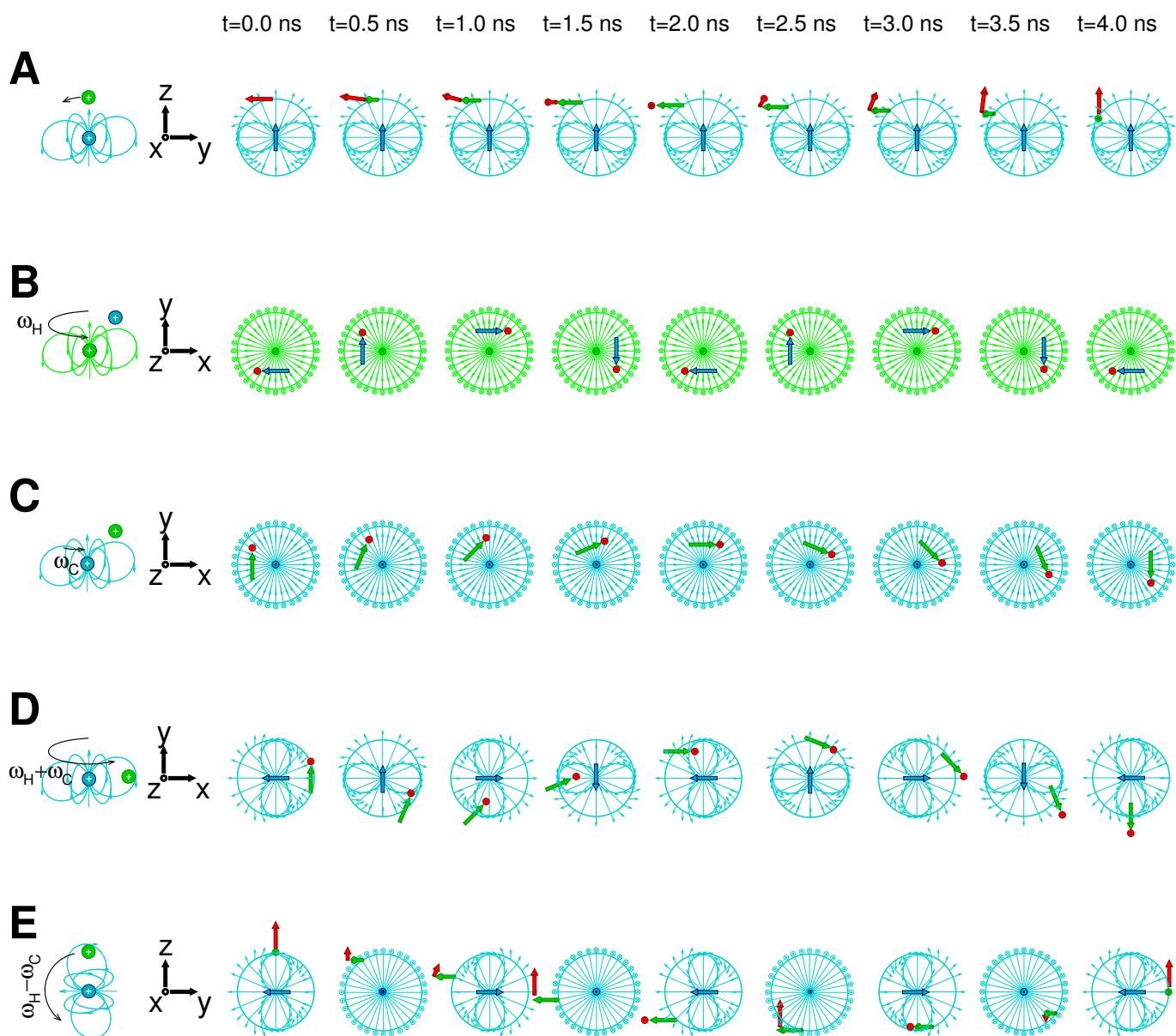
Figure 8.4: Illustration how random molecular motions resonating with five characteristic frequencies affect \vec{\mu}_C in the CH bond in a 500 MHz spectrometer ( \vec{B}_0 = 11.75 T). The first diagram in each row shows positions of the nuclei ( ^{13}\text{C} in green, ^1\text{H} in cyan), the second diagram shows orientation of the coordinate frame, the following diagrams are snapshots of the orientations of magnetic moments shown as arrows ( ^{13}\text{C} in green, ^1\text{H} in cyan) in a magnetic field of the neighbour (shown as force lines). The red arrow indicates the direction of the change of the orientation of the influenced magnetic moment, but the actual change is very small (not observable in the pictures) in the short depicted period of 4 ns. The molecule is assumed to rotate with a constant frequency for 4 ns. A, \vec{\mu}_C oriented horizontally, \vec{\mu}_H oriented vertically, ^{13}\text{C} in the yz plane, ^1\text{H} in the center of the coordinate system. Rotation at any frequency about a horizontal axis varies precession frequency of \vec{\mu}_C about \vec{B}_0 and results in the loss of coherence of ^{13}\text{C} . B, \vec{\mu}_H oriented horizontally, \vec{\mu}_C oriented vertically, ^1\text{H} above the xy plane, ^{13}\text{C} in the center of the coordinate system. Rotation at \omega_H about a horizontal axis pulls \vec{\mu}_H up (red arrow pointing up in the given coordinate frame) in the magnetic fields of \vec{\mu}_C . This reorientation of \vec{\mu}_H (observed only at time much longer than the depicted period of 4 ns) influences the effect of the J -coupling. C, \vec{\mu}_C oriented horizontally, \vec{\mu}_H oriented vertically, ^{13}\text{C} above the xy plane, ^1\text{H} in the center of the coordinate system. Rotation at \omega_C about a horizontal axis pulls \vec{\mu}_C up (red arrow pointing up in the given coordinate frame) in the magnetic fields of \vec{\mu}_H . D, \vec{\mu}_C oriented horizontally, \vec{\mu}_H oriented horizontally, ^{13}\text{C} in the xy plane, ^1\text{H} in the center of the coordinate system. Rotation at \omega_H + \omega_C about a horizontal axis pulls \vec{\mu}_C up (red arrow pointing up in the given coordinate frame) in the magnetic fields of \vec{\mu}_H . E, \vec{\mu}_C oriented horizontally, \vec{\mu}_H oriented horizontally, ^{13}\text{C} in the yz plane, ^1\text{H} in the center of the coordinate system. Rotation at \omega_H - \omega_C about a horizontal axis pulls \mu_C up (red arrow pointing mostly up in the given coordinate frame) in the magnetic fields of \mu_H . The reorientation of \mu_C in Panels C–E (observed only at time much longer than the depicted period of 4 ns) contributes to the return of the distribution of the ^{13}\text{C} magnetic moments to the thermal equilibrium.
