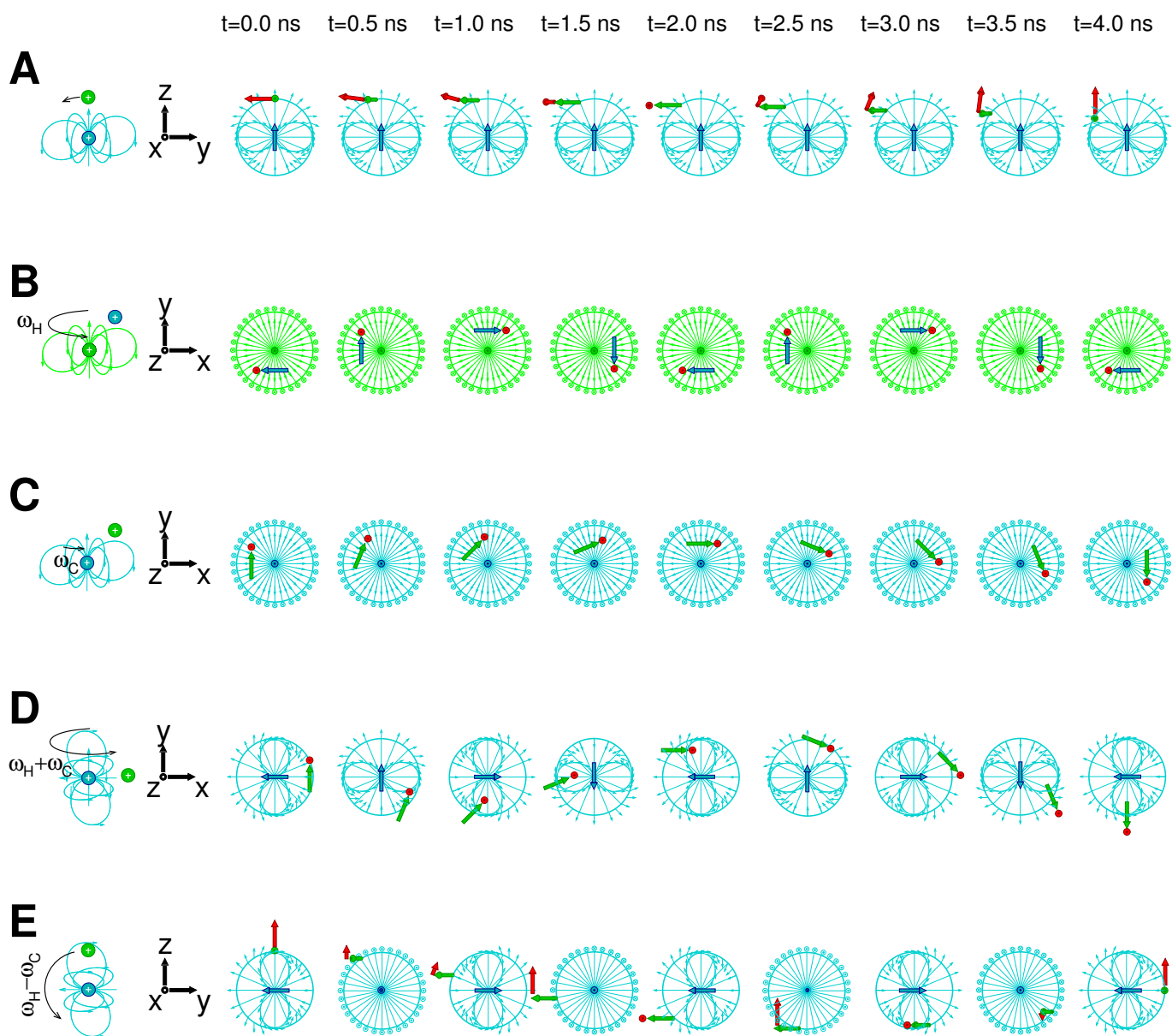
Figure 8.4: Illustration how random molecular motions resonating with five characteristic frequencies affect \vec{\mu}_C in the CH bond in a 500 MHz spectrometer ( \vec{B}_0 = 11.75 T). The first diagram in each row shows positions of the nuclei ( ^{13}\text{C} in green, ^1\text{H} in cyan), the second diagram shows orientation of the coordinate frame, the following diagrams are snapshots of the orientations of magnetic moments shown as arrows ( ^{13}\text{C} in green, ^1\text{H} in cyan) in a magnetic field of the neighbour (shown as force lines). The red arrow indicates the direction of the change of the orientation of the influenced magnetic moment, but the actual change is very small (not observable in the pictures) in the short depicted period of 4 ns. The molecule is assumed to rotate with a constant frequency for 4 ns. A, \vec{\mu}_C oriented horizontally, \vec{\mu}_H oriented vertically, ^{13}\text{C} in the yz plane, ^1\text{H} in the center of the coordinate system. Rotation at any frequency about a horizontal axis varies precession frequency of \vec{\mu}_C about \vec{B}_0 and results in the loss of coherence of ^{13}\text{C} . B, \vec{\mu}_H oriented horizontally, \vec{\mu}_C oriented vertically, ^1\text{H} above the xy plane, ^{13}\text{C} in the center of the coordinate system. Rotation at \omega_H about a horizontal axis pulls \vec{\mu}_H up (red arrow pointing up in the given coordinate frame) in the magnetic fields of \vec{\mu}_C . This reorientation of \vec{\mu}_H (observed only at time much longer than the depicted period of 4 ns) influences the effect of the J -coupling. C, \vec{\mu}_C oriented horizontally, \vec{\mu}_H oriented vertically, ^{13}\text{C} above the xy plane, ^1\text{H} in the center of the coordinate system. Rotation at \omega_C about a horizontal axis pulls \vec{\mu}_C up (red arrow pointing up in the given coordinate frame) in the magnetic fields of \vec{\mu}_H . D, \vec{\mu}_C oriented horizontally, \vec{\mu}_H oriented horizontally, ^{13}\text{C} close to the z axis, ^1\text{H} in the center of the coordinate system. Rotation at \omega_H + \omega_C about a vertical axis pulls \vec{\mu}_C up (red arrow pointing up in the given coordinate frame) in the magnetic fields of \vec{\mu}_H . E, \vec{\mu}_C oriented horizontally, \vec{\mu}_H oriented horizontally, ^{13}\text{C} in the yz plane, ^1\text{H} in the center of the coordinate system. Rotation at \omega_H - \omega_C about a horizontal axis pulls \mu_C up (red arrow pointing mostly up in the given coordinate frame) in the magnetic fields of \mu_H . The reorientation of \mu_C in Panels C–E (observed only at time much longer than the depicted period of 4 ns) contributes to the return of the distribution of the ^{13}\text{C} magnetic moments to the thermal equilibrium.
