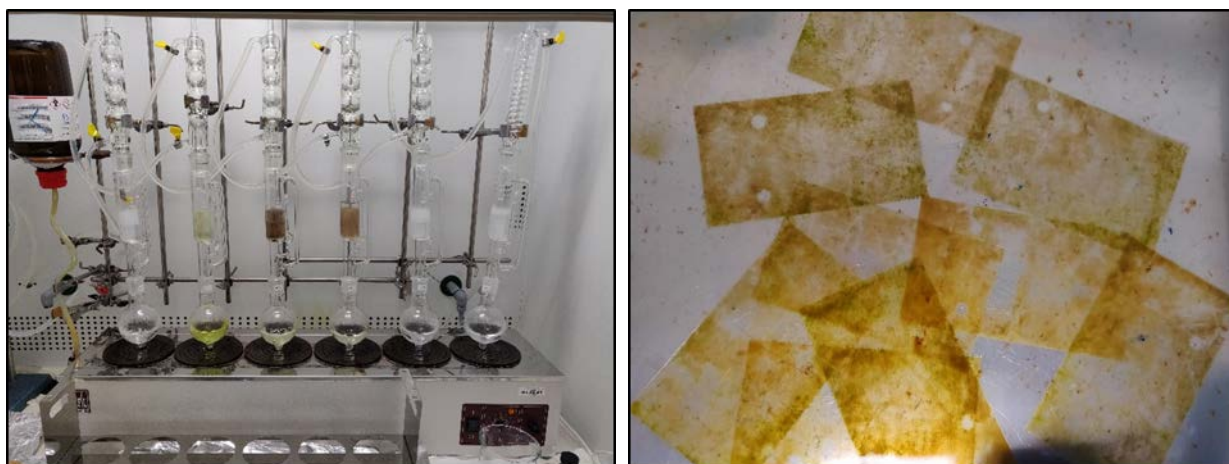
Figure 2: Left – Apparatus for extraction of silicone rubbers – 250mL point flask, Soxhlet with accordion folded silicone rubbers, cooler. Right – Uncleaned silicone rubbers after exposure.
