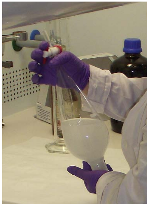
Figure 1 Shaking and simultaneously releasing gases
