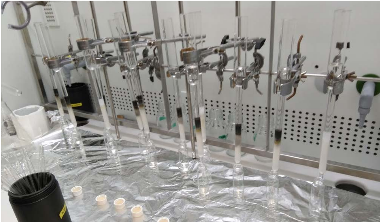
Fig. 5: Column chromatography with sulphuric acid-modified silica gel
