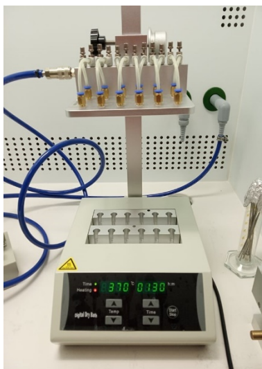
Figure 1 Equipment for enzymatic incubation (37 °C, 90 minutes)
