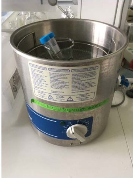
Figure 1 and 2 – Extraction of soil sample in ultrasonic bath
