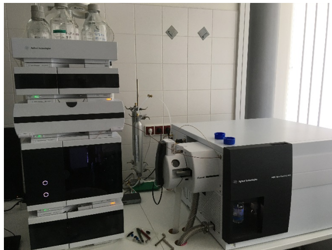
Figure 4 – Liquid chromatography coupled with tandem mass spectrometry
