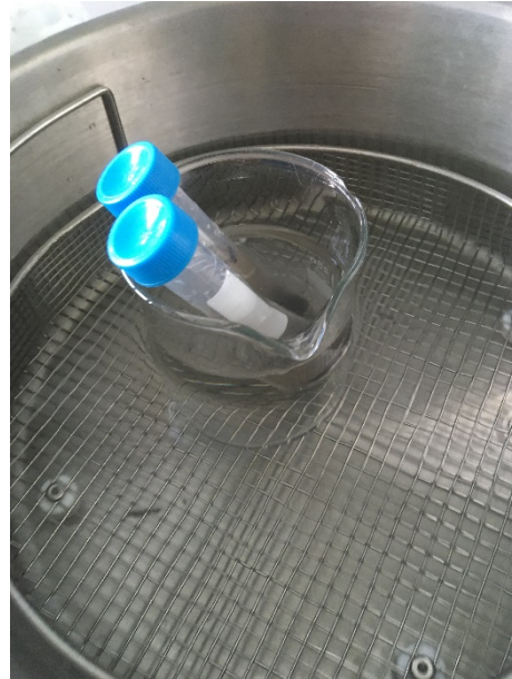
Figure 1 and 2 – Extraction of soil sample in ultrasonic bath
