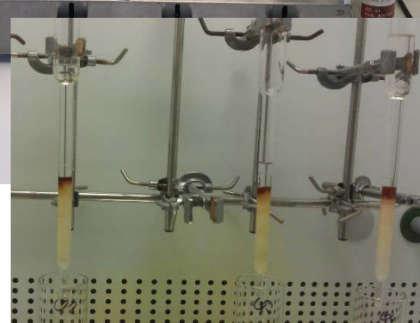
Picture 3 Photo of cleaning columns
