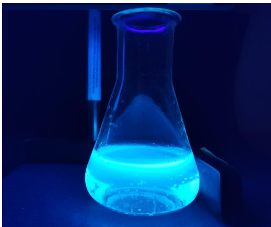
Obr. 28: Fluorescence chininu v toniku
