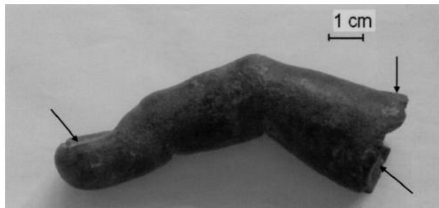
Fig. 2. Fragment of Roman sculpture: the areas analyzed by LIBS are shown by arrows.
