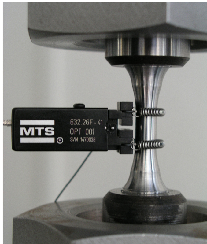
Figure 2.15 a), b) Schematics of tensile test machines. c) Servohydraulic machine, d) specimen for the fatigue test with attached extensometer.
