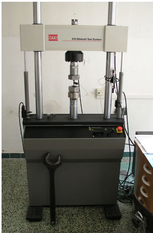
Figure 2.15 a), b) Schematics of tensile test machines. c) Servohydraulic machine, d) specimen for the fatigue test with attached extensometer.
