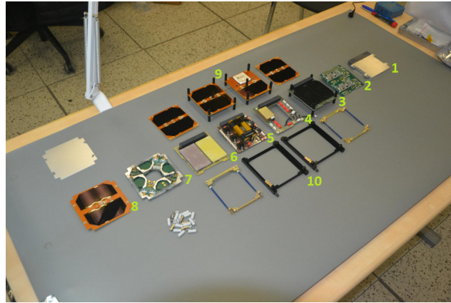
Figure A.6: Internal components of the GRBAAlpha satellite. 1. Scintillator; 2. electronics; 3. onboard computer + GPS; 4. Lodestone and X-ray detector (X-ray dosimeter from VZLÚ); 5. power supply module with batteries; 6. UHF and VHF transceiver; 7. antenna mount; 8., 9. solar panels; 10. frames (Pál et al. 2020).
