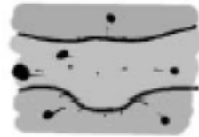
(e) Post-discharge : solidifying and flushing of the eroded particles by the dielectric
