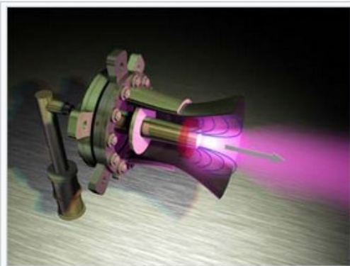
CGI rendering of Princeton University's lithium-fed self-field MPD thruster (from Popular Mechanics magazine)
