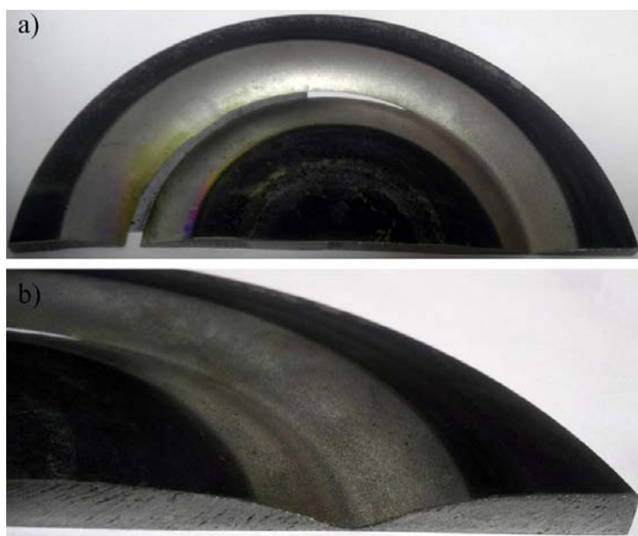
Figure 1.3: Racetrack formed throughout the target life. a) top view b) side view
