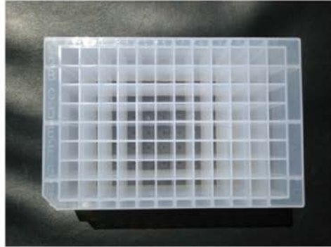
96-well deep plate for purification
