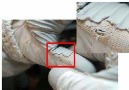
(d) Damage on astronaut mastracchio's left glove due to a crater lip on the ISS's handrails
