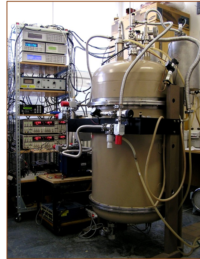
ConEV apparatus (Rayleigh-Bénard convection)
