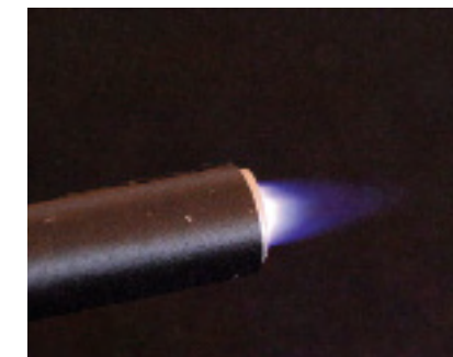
Plasma needle - atmospheric plasma - analysis with EQP/HPR 60 molecular beam sampling system.
