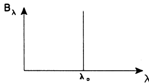
Recorded spectrum of a monochromatic light source with a perfect instrument.
