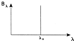
Real spectrum of a monochromatic light source.
