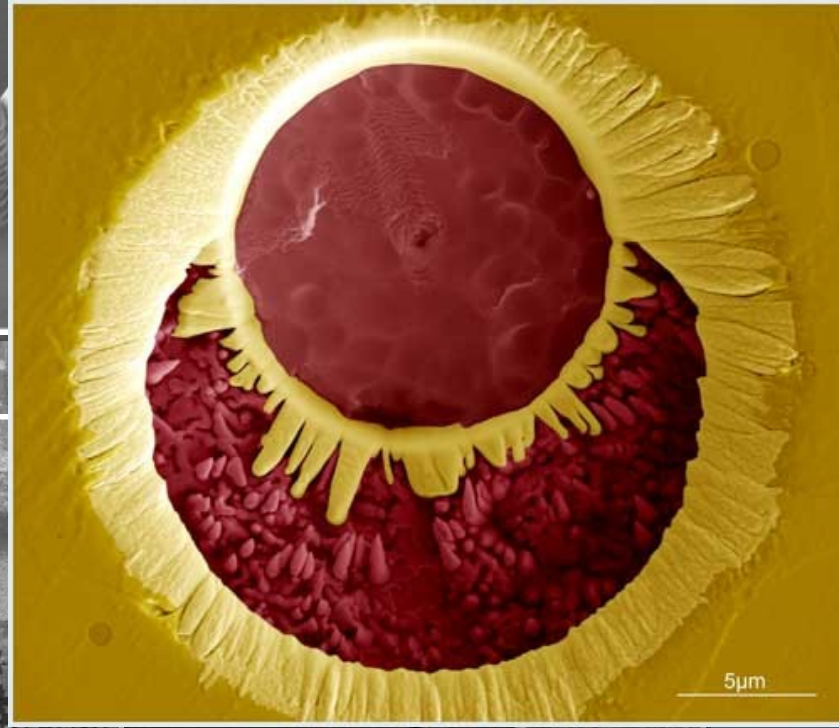
FIB-cut in steel v2a FF by 1nA to 1µm milling-002 steel water imaged with a plasma FIB
