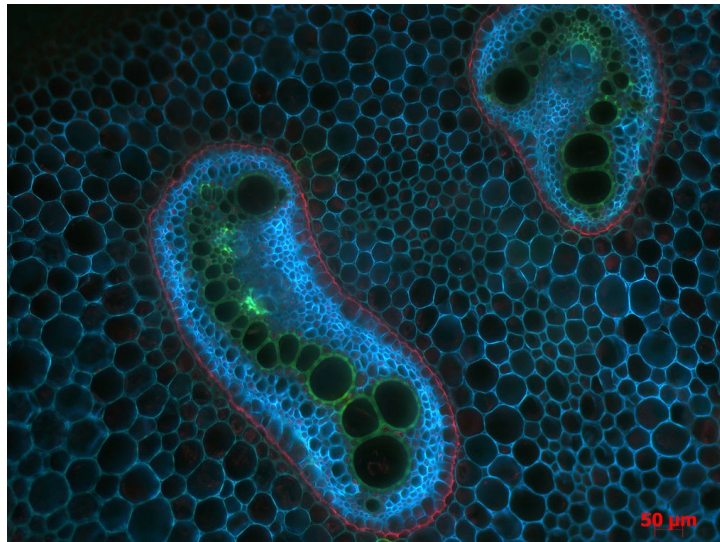
Fig 2. Combined red and green channel confocal images of acridine orange -stained spruce early wood. The staining conditions were 50 \mu\text{mol/L} acridine orange in phosphate buffer, pH 7. The scale bar is 100 \mu\text{m} .
