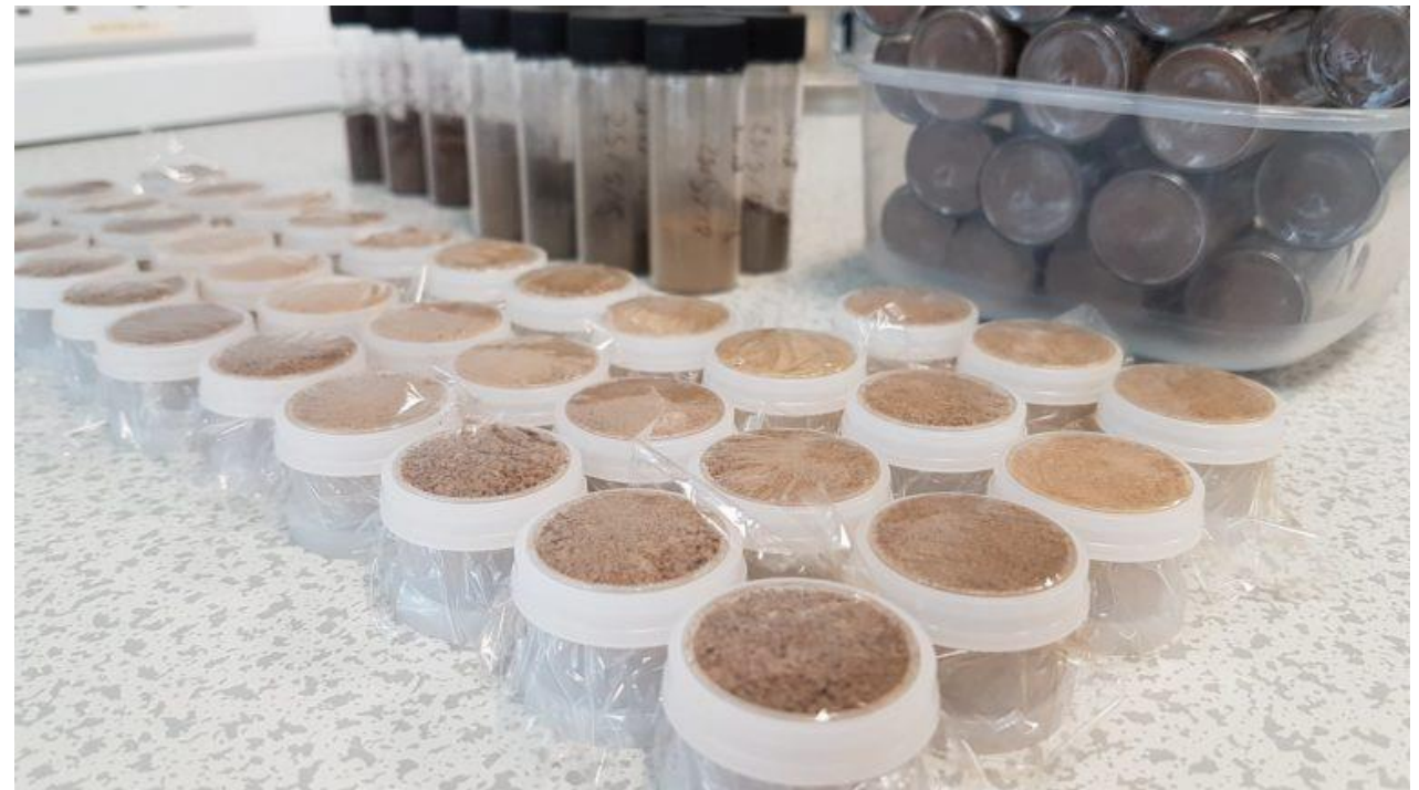
Powdered bone and soil samples to test for chemical element composition using XRF.
