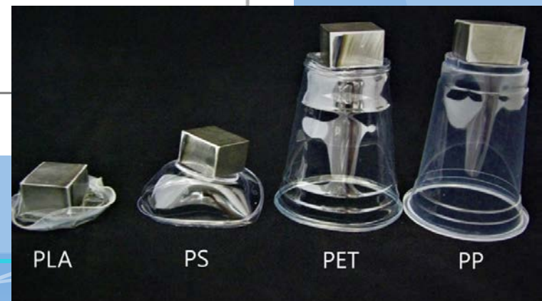
Figure 6 - Deflection under 0.31lb at 160°F
