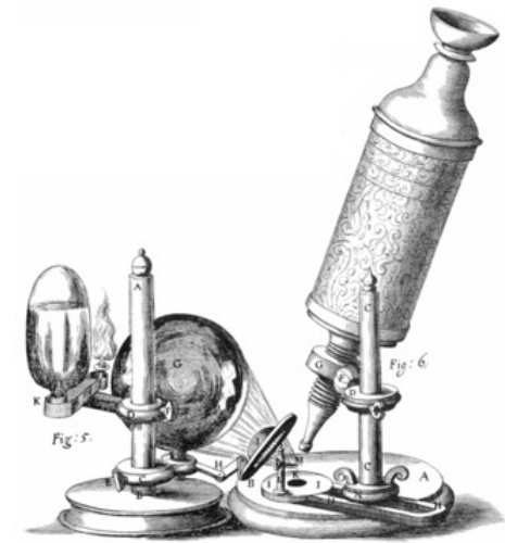
Hooke-microscope Hooke was an early one to build and experiment with microscopes
