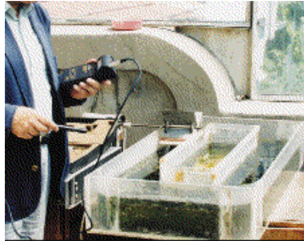
Figure 4.2 FIFRA microcosm experimental unit. An example of a microcosm experimental unit designed to test the effects of a herbicide on an aquatic environment. This particular setup does not include fish since the predatory effects would tend to hide lower trophic level effects upon the invertebrate populations. Typically, a FIFRA microcosm experiment includes fish species, particularly when acetylcholinesterase inhibitors or other toxicants particularly effective against animal species are tested.
