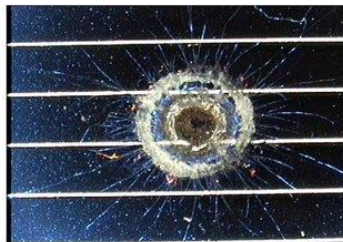
(a) Impact on a Hubble Space Telescope (HST) solar cell. Diameter, d=2.4 mm
