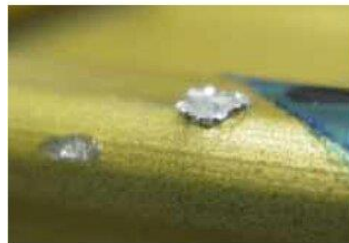
(c) Largest crater found on the handrails of the ISS. Diameter, d=1.85 mm and 0.33 mm-high crater lips
