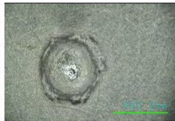
(b) Largest crater found on the International Space Station (ISS) airlock panels. Diameter, d=1.8 mm
