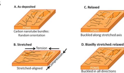
Revolution of morphology of films of carbon nanotubes with: (a) stretching; (b) under strain; (c) stretched and released along one axis; (d) and stretched and released along two axes.
