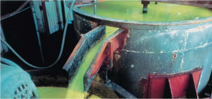
Figure 16.4 Ammonium diuranate (yellowcake) after solvent extraction. (Photo courtesy of UIC.)
