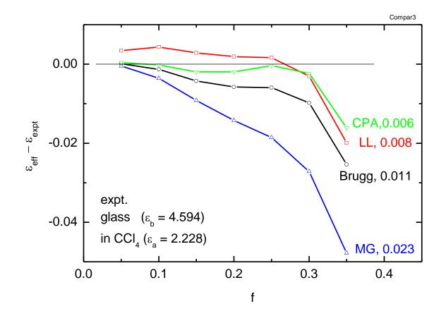
The typical use of EMA is an estimation of the volume fractions
