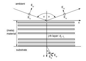
electric field inside the superlattice of absorbing/dielectric materials
