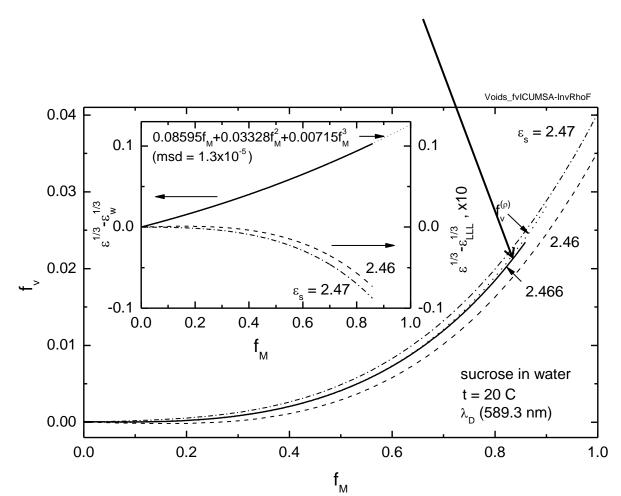
Fairly good agreement of optical data with EMA for the very small volume of the sugar molecule (0.35 nm<sup>3</sup> at RT) !
