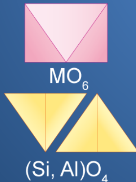
kaolinit \text{Al}_2(\text{OH})_4\text{Si}_4\text{O}_{10} (dioktaedrický) serpentín \text{Mg}_3(\text{OH})_8\text{Si}_4\text{O}_{10} (trioktaedrický)
