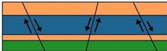
2. Layers are cut by normal faults
