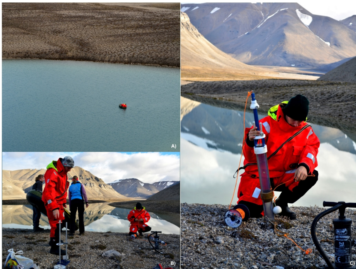
Figure 4 (a): Search for the core's retrieval point in the Lake Mathiesondalen 3; (b): Field coring preparation (surrounding/background slopes formed mainly by dolomite, limestone and gypsum); (c): Gravity corer used for extraction (all photographed on 21/08/2015 by Matěj Roman and Jan Kavan).
