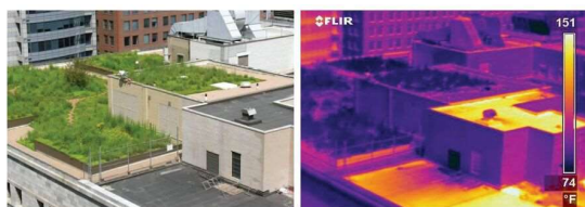
On a typical day, the Chicago City Hall green roof measures almost 80°F (40°C) cooler than the neighboring conventional roof.
