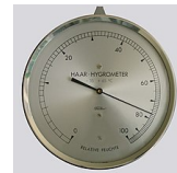
A hair tension dial hygrometer
