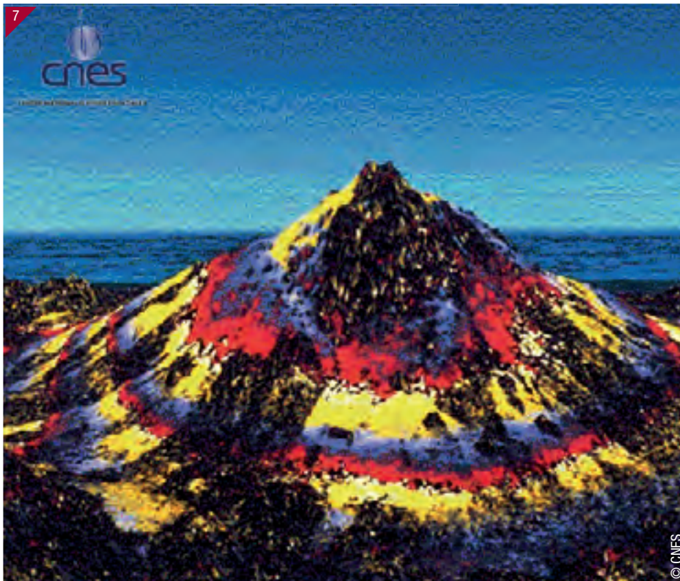
In this image one can see four series of concentric coloured bands. Each cycle represents a 2.8 cm elevation of the volcano in the direction of the satellite. This shows that the summit of Mount Etna has risen temporarily by 11.2 cm.
